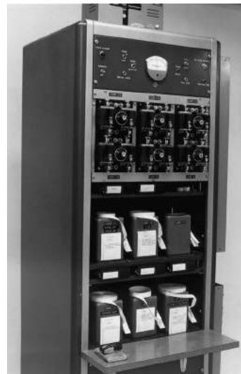
Alarm photos by R.K. Sunderbruch thought to have been taken in 1969. McCullough Register with Pony Packs series loop telephone circuitry service customers and Morse code-like boxes for every customer.
